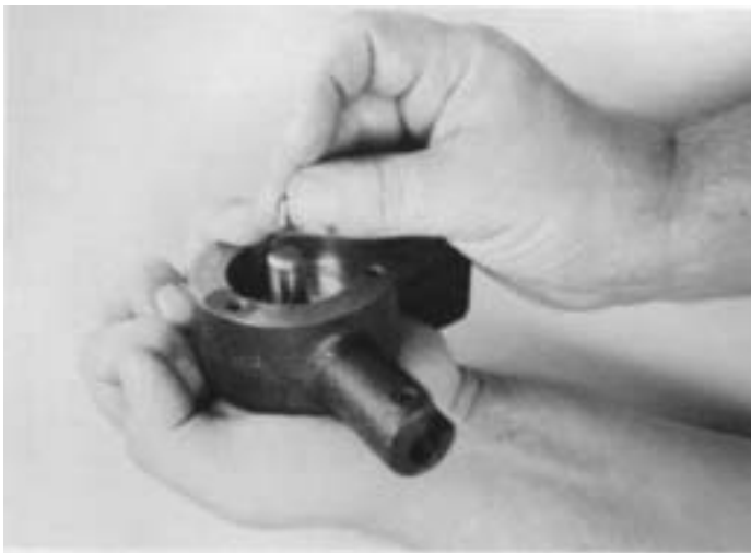
11. Remove two keys from drive shaft keyways.
