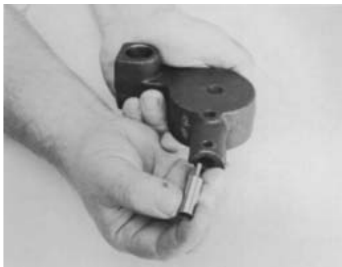
14. Remove relief valve from housing bore.
