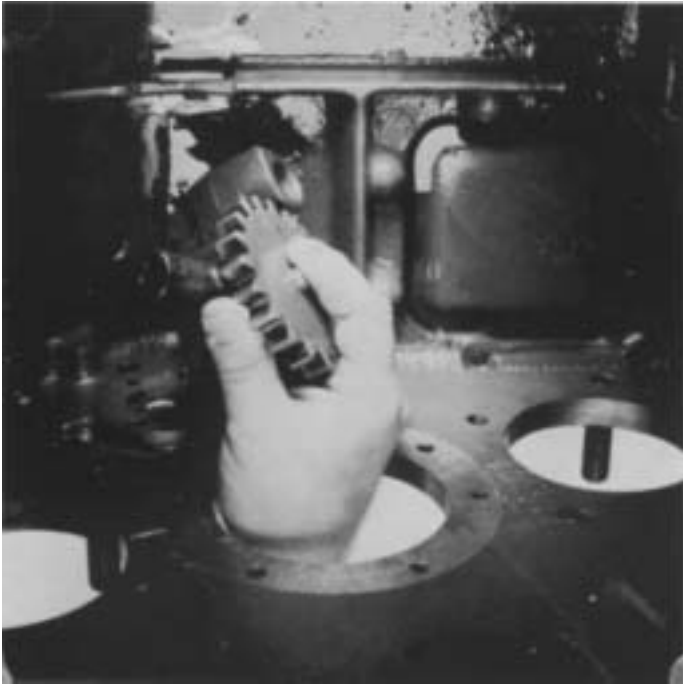
3. Remove the integral oil pump from case.
