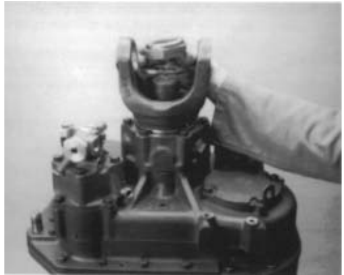
3. Install washer and output nut onto the output shaft.
