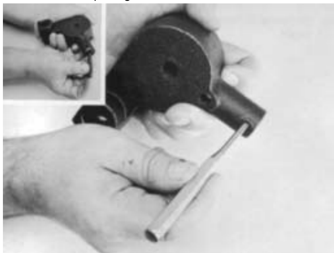
13. Remove relief valve roll pin from pump housing, relief valve spring can now be removed from relief valve housing bore (inset).
