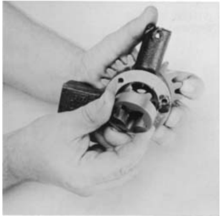
5. Remove outer oil pump element from pump.
